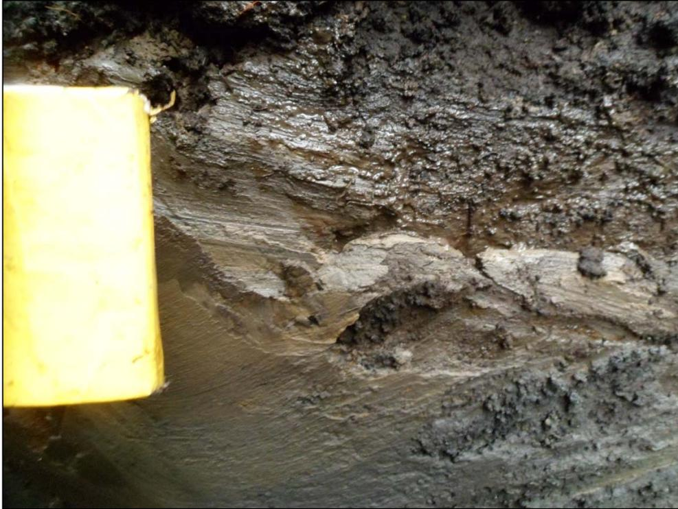
Photo 5 Underlying soft silt/clay at trial pit TP3
