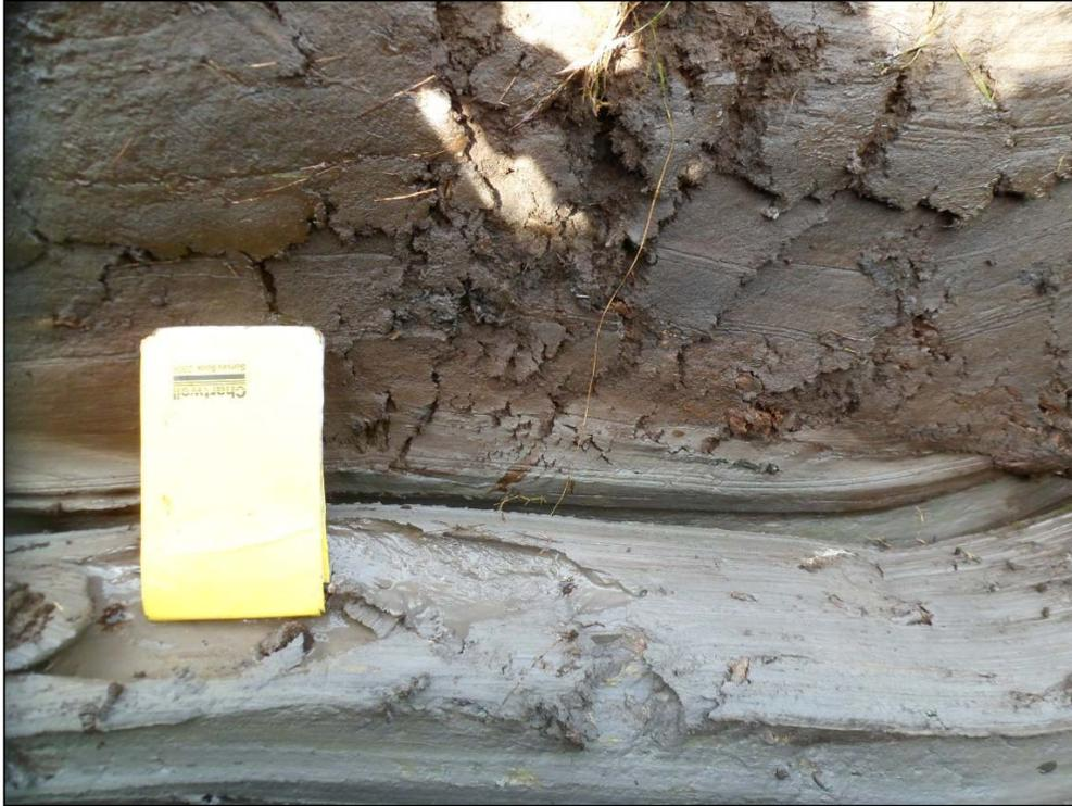
Photo 3 Underlying soft silt/clay at trial pit TP2
